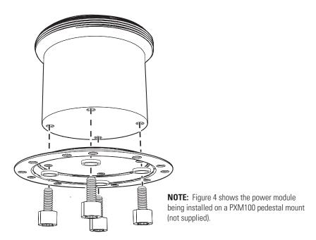
Figure 4. Attach Power Module to PXM100
